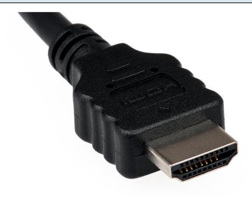
This is an HDMl plug. If your laptop has an HDMl port instead of a VGAport, you will need an HDMl-to-VGAadapter.
